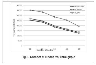
In fig.3 AODV and AOMDV show similar variations of throughput for varying number of nodes. Overall, AntHocNet shows highest throughput and outperforms the other two. The average throughput degrades the performance of large scale networks on account of congestion in the large scale networks.
