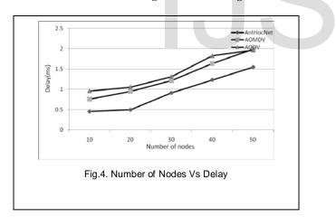
The term end-to-end delay does not have much significance in this scenario. The performance of AOMDV is slightly better than AODV especially when the number of nodes cross 30 due to stable maintenance of routing table. AntHocNet produces lower delay due to the fact that it uses different path scheme in the route reply.
